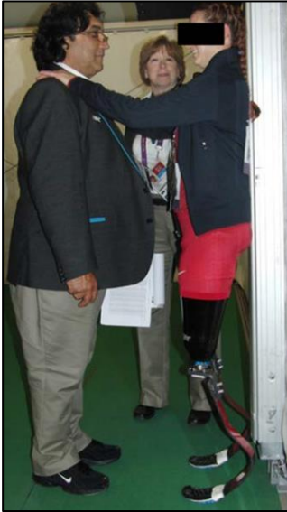
Figure 2: Athlete standing against a rigid pole, rather than a wall, which allows the most posterior part of the blades to be positioned behind the pole
